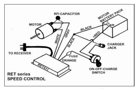
Connect the motor to the controller's white and gray heavy gauge wires. If throttle stick operation is backwards simply reverse these two motor wires; do *NOT* reverse the battery connections.
