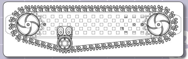
You need to build (2x) modules; one like the one above, and a mirrored version for the other side. After both modules are fully assembled, you can loosen the mounting screws, and slide the Idler Wheels until the Tank Tread is tensioned well. The tread should be tight, and only have a little bit of flex up and down.
