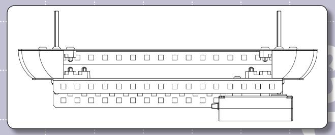
First install a Shaft Collar on each of the shafts, against the drive module chassis. (You will need to use the Shaft Collars that you previously removed from VEXplorer drive module.)
