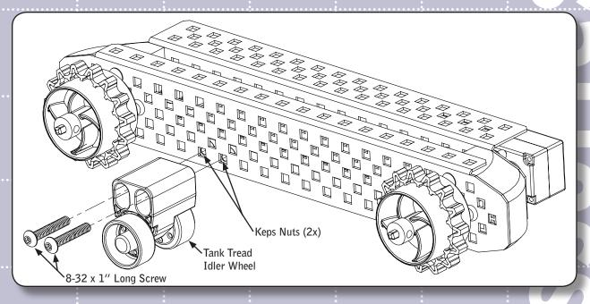
This Idler Wheel has mounting "slots" in it. These slots allow for tensioning of the Tank Treads. These can be arbitrarily set now, and adjusted later.
