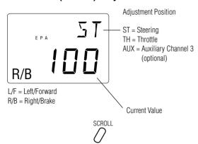
**1.** From the Servo Reverse function, press the *Scroll* key four times to access the End-Point (Travel) Adjustment function (the EPA screen with "ST" will appear).
