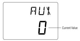
When the LN (linear) Auxiliary Channel 3 function is selected, Grip Lever A can be used to change the neutral position of the servo to lean or richen the engine's fuel mixture. Once the desired fuel mixture has been achieved, the Grip Lever A value indicated on this screen can be transferred manually to the Sub-Trim function and the value of the AUX screen can be returned to zero. Please refer to diagram A below for proper grip lever operation.
