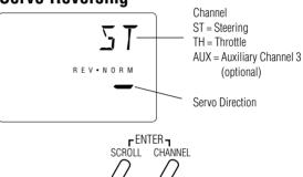
**1.** With the transmitter power switch on, press the *Scroll* key to enter the Function mode.
