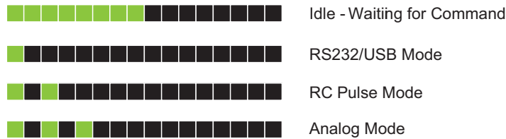
FIGURE 8. Normal Operation Flashing Patterns
