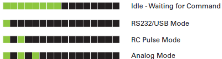
FIGURE 11. Normal Operation Flashing Patterns
