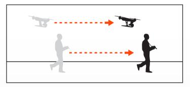
**Important Note:** In Follow Me function, the aircraft will maintain a constant altitude and cannot detect obstacles. Pilots who change their altitude by for example, moving to higher ground, during flight should be mindful of this.
