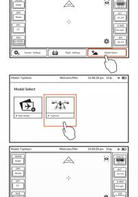
**Step 2)** Tap the 'Model Select' button, and if required press 'OK' to bypass any pop up warnings/alerts.
