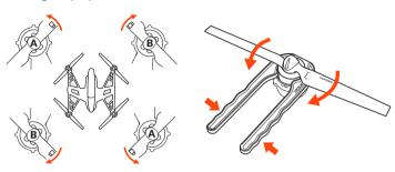
Each motor and propeller are marked with an 'A' or 'B' to ensure easy installation in the correct positions (for example: install propellers marked with 'A' on motors marked with 'A').
