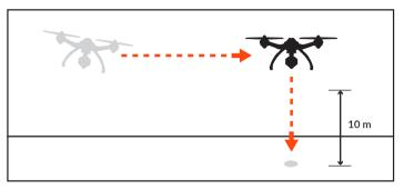
**B)** When flying lower than 33 feet (10 meters) the TYPHOON will climb to 33 feet (10 meters) while flying back to the home point, or active home position, then descend vertically until it lands.
