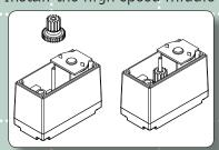
7. Install the output bushing removed in step 3. Make sure the bushing orientation is as shown.
