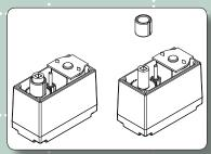
5. Install the high speed middle gear.
