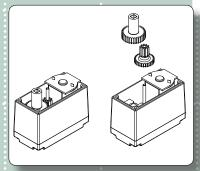
6. Install the high speed output shaft gear.
