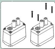
3. Lift off the output bushing and place to the side. This will be used later.
