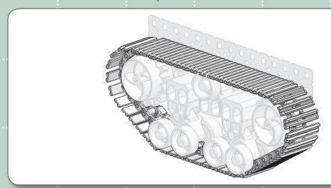
You can now slightly loosen the screws holding the bogey wheel assemblies and tensioner in place. Slide the tensioner and the bogey wheel assemblies to tighten the chain of tread links. If the tread links are loose, they'll come off once the robot is in motion.
