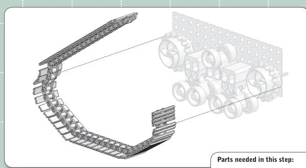
Note how the teeth on the drive wheel fit between the rollers on the tread links.
