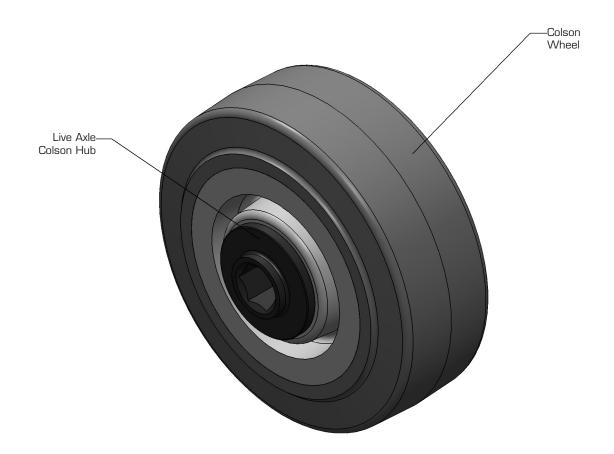
Note: The Colson Live Hub is designed to be pressed into the bore of Colson Performa Wheel. There is a .0125" interference fit between the hub and bore of the Colson Wheel. This will require an arbor press or large vise to assemble. It is NOT recommended to hammer the hub into the bore, as this can lead to damage and misalignment between the hub and wheel.
