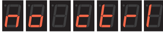
FIGURE 81. "No control" message will scroll when no valid radio signal is present
