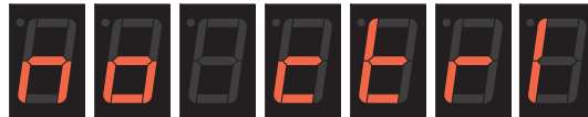
FIGURE 87. The “no control” message indicates that joystick is not centered at power up
