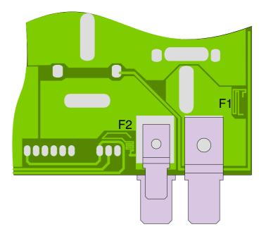
Do not use a strand thicker than 0.2mm diameter as this could allow other tracks to get damaged in the event of a fault. This may make the controller unrepairable.
