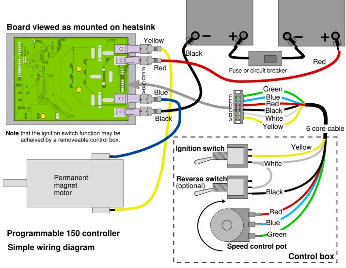
The diagram shows the simplest wiring for the Pro-150. Wiring is covered in more detail in section 5.1.
