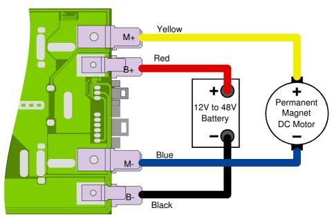
If the motor has a higher current rating than the controller, the full torque output of the motor will not be available, but the controller will not be damaged since the motor current is automatically limited to a safe value for the controller.
