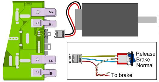
A 3rd pin (C) is present: this is internally connected to battery -ve and may be used to wire a 3 position switch as show inset.
