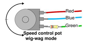
If this resistor is not fitted a fault such as a break in the top of the pot or a short wiper to battery -ve will not be detected and may cause full speed operation.
