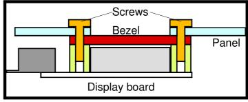
If you apply a thin bead of silicone rubber behind your panel before mounting the display you can easily make this completely water tight.
