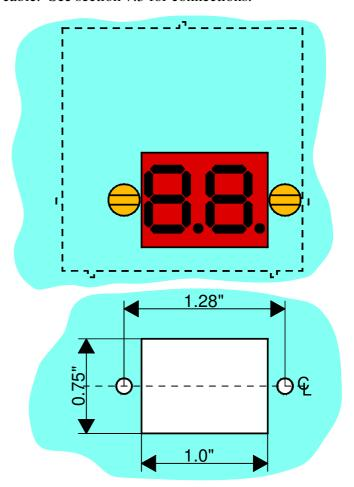
The display requires a rectangular cut-out in your panel, with two M3 clearance holes as shown above.
