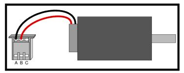
drive such a brake: power is applied to the solenoid as demand speed is increased above zero and when the demand speed returns to zero, power is removed. Parking brake drive is via the 3 pin connector, shown on the diagram 'Features'. This should be wired as in the first diagram.
