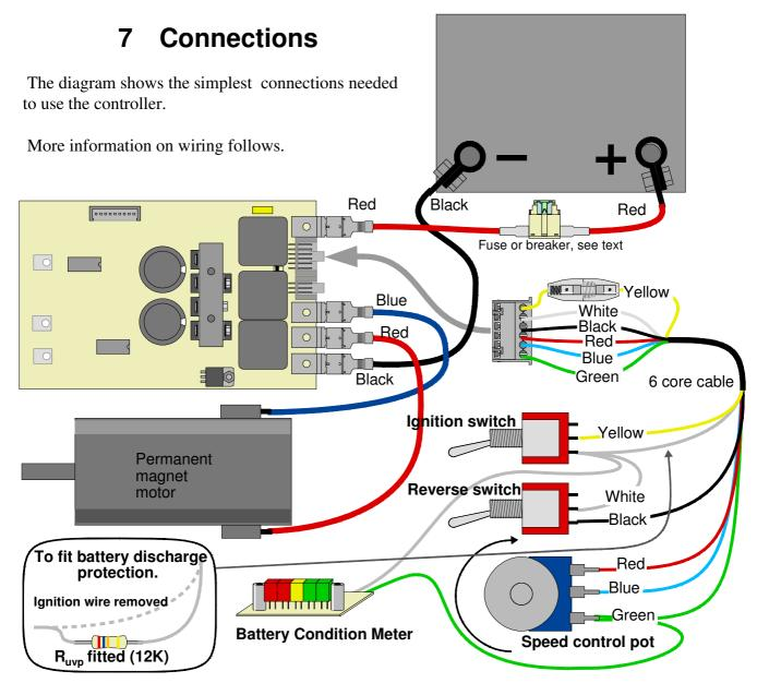
Yellow is directly connected to battery +ve. White and black may also be battery +ve (depending on the control switches). Green is battery -ve and blue and red are the control pot.
