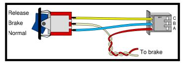
The 3rd pin is battery negative so you can use a 3 position switch to give Release—Brake—Normal (brake override facilities), as shown in the diagram below.
