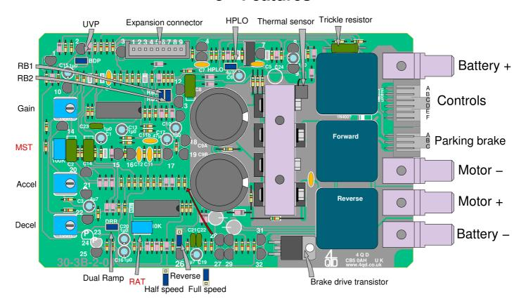
For shipping, the mating parts of the 'Controls' and 'Parking brake' connectors are inserted into the sockets on the board. See page 7.
