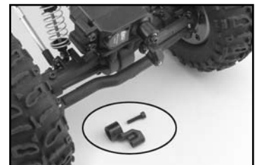
3. With servo output shaft still centered, install solid servo arm with the shorter screw supplied and attach steering linkage.
