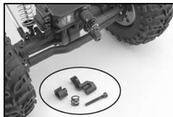
2. Remove servo saver arm assembly from the servo. Remove the steering ball stud and install into solid servo arm.
