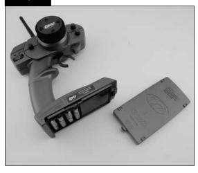
Remove the transmitter battery cover by sliding the cover from left to right. Install four (4) AA batteries into the battery holder. Pay close attention to the correct direction of the positive (+) and negative (-) ends as marked in the tray. Once all 4 batteries have been installed, reinstall the battery cover by sliding it on from right to left.
