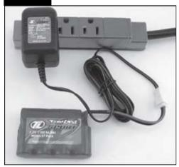
Plug the AC charger into the proper wall receptacle (110V). Plug the battery pack into the charger and let it charge for 3 hours for the first time. After running, or when the Mini-Rock Crawler slows noticeably, recharge the battery pack for 5 to 6 hours for a full charge.
