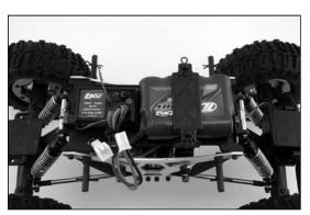
Install the charged battery pack into the chassis as shown (fig.2). Ensure that the battery is laying flat on the chassis.
