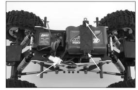
Reinstall the battery strap and body clips. Plug the battery pack into the ESC (fig. 3).
