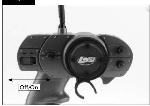
Always turn on the transmitter first by sliding the switch on the left side of the wheel from left to right. The small red and green lights above the switch should both light up. If not, you need to check for low or incorrectly installed batteries.
