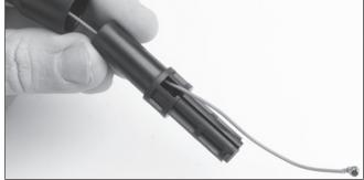
12X - Reassemble the new antenna assembly and the shaft. Routing the coaxial wire through the shaft until the coax wire exits the opening at the base of the shaft. Align housing with the antenna shaft until the Phillips head screw holes line up. Avoid pinching the antenna wire. Install the Phillips head screw.
