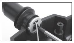
**12X** - Install the antenna mount assembly in the transmitter routing the coaxial antenna wire through the hole in the board to reach the RF module.
