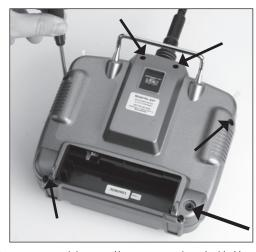
**12X** - Remove rear module cover. Use care to not lose the bind button extension.
