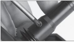
**12X** - Using a 2.5mm hex driver remove the 4 screws holding the transmitter top onto the case.
