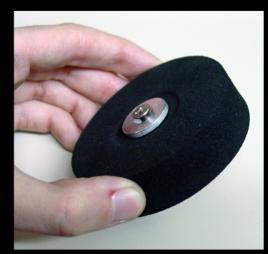
Insert the screw through the small piece you just aligned and thread it into the hub on the other side. Tighten it down using a screwdriver.
