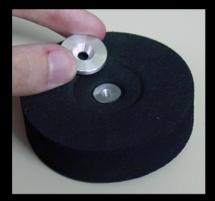
Now flip the wheel over and align the other half of the hub with the larger piece.
