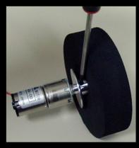
Insert the hub onto your motor's output shaft. Tighten down the set screw (preferably onto the shaft's flat, if there is one).
