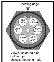
The diagram, left, shows the pin connections on the 6 way connector commonly used with our controllers.
