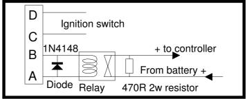
When the battery is connected up, current flows through the resistor to charge up the controller's capacitors. When the ignition is switched on, the capacitors are connected across the relay coil which pulls in, shorting out the resistor. If the battery is reversed the MOSFETs in the controller short out the capacitors so they do not charge up and the relay cannot operate. The fault current is limited by the resistor to a safe value.
