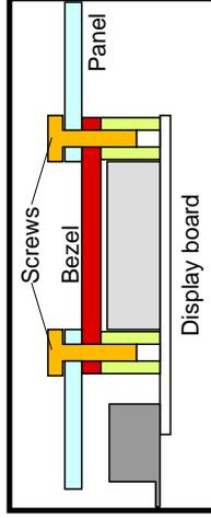
If you apply a thin bead of silicone rubber behind your panel before mounting the display you can easily make this completely water tight.
