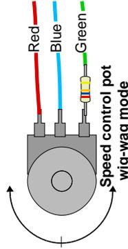
If this resistor is not fitted a fault such as a break in the top of the pot or a short wiper to battery - we will not be detected and may cause full speed operation.
