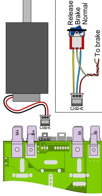
The controller does not detect an open-circuit parking brake so this may be left disconnected if a brake is not fitted.
