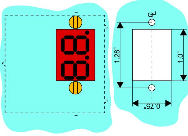
The display requires a rectangular cut-out in your panel, with two M3 clearance holes as shown above.
