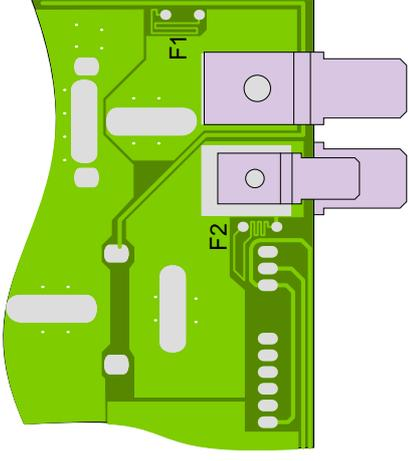
*Do not use a strand thicker than 0.2mm diameter as this could allow other tracks to get damaged in the event of a fault.*
