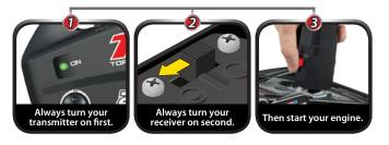
In order for the transmitter and receiver to bind to one another, the receiver in the model must be turned on within 20 seconds of turning on the transmitter. The transmitter LED will flash fast red, indicating a failure to link. If you miss it, simply turn off the transmitter and start over.
