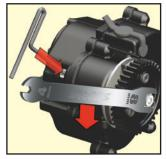
end of the slipper shaft. This locks the shaft for adjustments. Turn the adjustment nut clockwise to tighten (less slippage) and counter-clockwise to loosen (more slippage). The slipper clutch has two functions:
