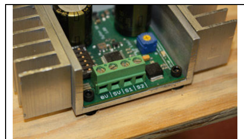
Figure 2.3: Mounted to a wood frame using standoffs
