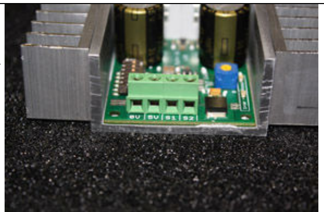
The input signal connects to terminal S1 and sometimes S2
