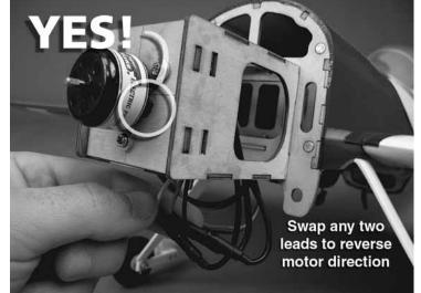
4. Mount your motor to the firewall using the screws, washers, and blind nuts supplied with your model kit. 4-40 sized hardware or 3mm hardware is adequate for these SuperTigre motors. If you are using the SuperTigre 370 or 400 motor, route the motor
