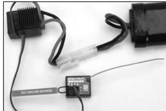
Powering the receiver with an ESC
