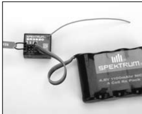
Powering the receiver with a separate receiver pack
