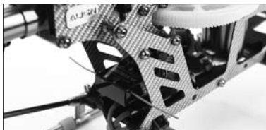
AR6115 installed in Heli
