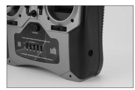
A charging jack is located on the right side of the transmitter. If rechargeable batteries are used they can be conveniently charged without removing them from the transmitter using the charge jack.
