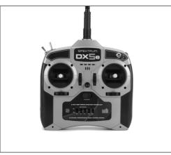
4. Pull and hold the trainer switch on the top of the transmitter while turning on the power switch. Release the trainer switch once the LEDs on the front of the transmitter flash, and a series of tones are heard. Within a few seconds the system should connect. Once connected the LED on the receiver will go solid indicating the system is connected.
