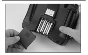
Remove the battery door and install 4 AA batteries. Make sure the polarity of each corresponds with the diagram in the battery holder. Replace the battery door.
