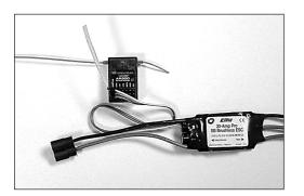
**Note**: To bind an aircraft with an electronic speed controller that powers the receiver through the throttle channel (ESC/BEC), insert the bind plug into the BATT/ BIND port in the receiver and the throttle lead into the throttle port. Proceed to Step #2. 2. Power the receiver by plugging in a receiver battery in any port on the receiver. Note that the LED on the receiver should be flashing, indicating that the receiver is in bind mode and ready to be bound to the transmitter.
