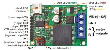
Pololu jrk 12v12 USB motor controller with feedback, labeled top view.
