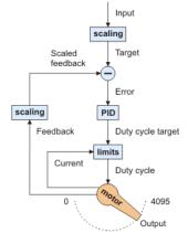
Diagram of a typical feedback system, showing quantities computed by the jrk.
