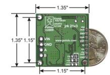
Pololu jrk 21v3 USB motor controller with dimensions.
