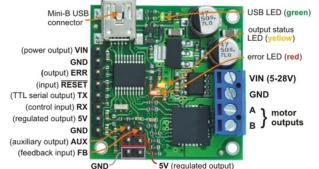
Pololu jrk 21v3 USB motor controller with feedback, labeled top view.
