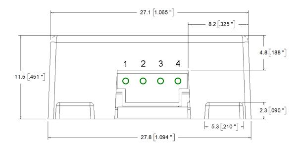
Part number A98655-ND from Digi-Key is a compatible connector for the 4-pin side output of the sensor (compatible connecting cables are also available from CH Robotics).
