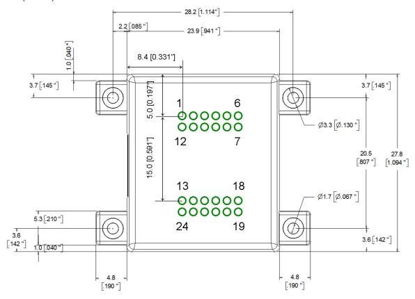
Part number 609-2890-ND from Digi-Key is a compatible 2mm pin header for connecting to the bottom connectors on the UM6.
