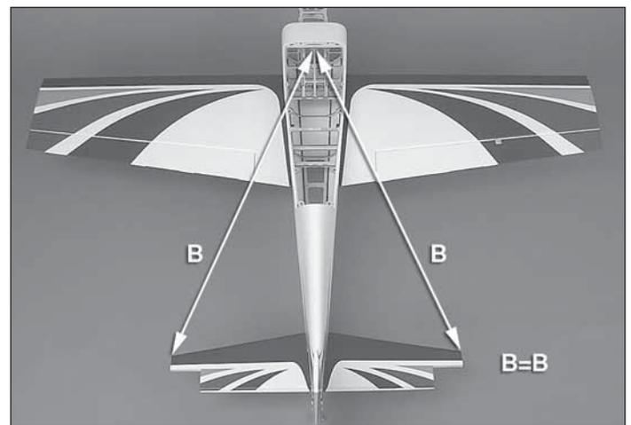
3. Measure the distance from the tip of the stab to the center of the fuselage. Adjust the position of the stab until they are equal. The stringer is centered in the front of the fuselage.
