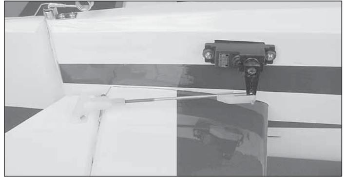
❑ 5. Slide a silicone clevis retainer over the clevis. With the elevator servo and the elevator centered, mark the elevator pushrod where it crosses the elevator servo arm. Make a 90° bend at the mark. Cut the pushrod 3/8" [9.5mm] past the bend. Attach the pushrod to the elevator servo arm with a nylon FasLink.
