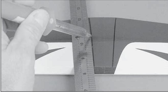
Use a straightedge to guide the soldering iron at a rate that will just melt the covering and not burn into the wood. The hotter the soldering iron, the faster it must travel to melt a fine cut. Peel off the covering.
