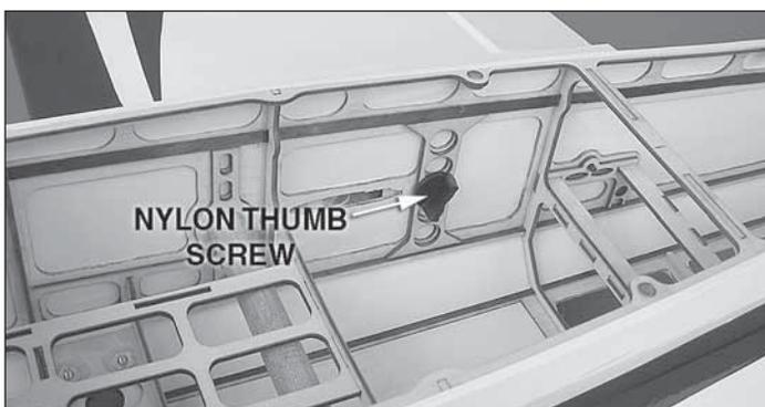
1. Center the wing tube in the fuselage. Slide the wing halves onto the wing tube and secure the wing halves to the fuselage with the nylon 10-24 thumb screws. Be careful putting pressure on the wing and fuselage. The wings may be tight the first time they are slid on the tube.
