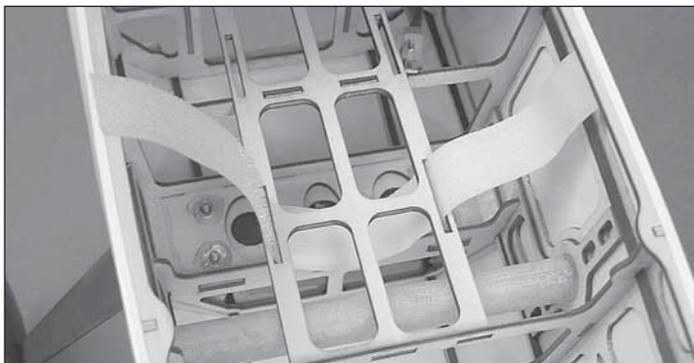
❑ 8. Overlap by 1" [25mm] two strips of non adhesive backed hook and loop material. Route the hook and loop material
