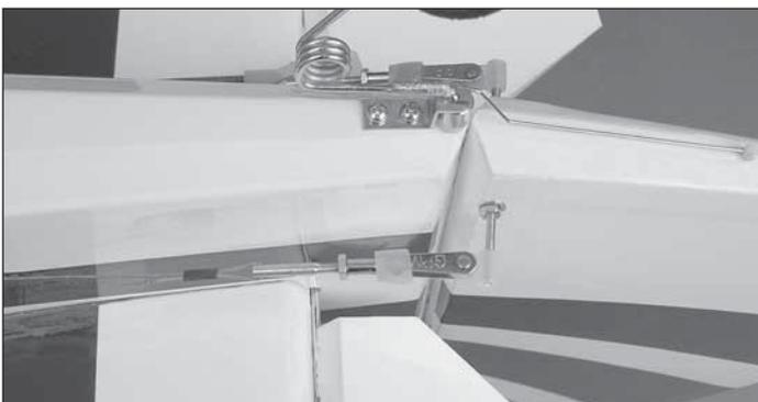
❑ 10. Pull the pull-pull string out of the fuselage aft end so that the string is tight. Pass the string through a crimp, through the rigging coupler and back through the crimp. Attach the clevis to the nylon torque rod horn on the rudder and tape the string to the side of the fuselage. Repeat on the other side of the fuselage.
