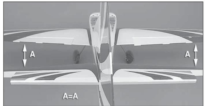
2. Center the horizontal stabilizer in the slot in the fuselage. Stand back and look at the stab in relation to the wing. The stab should be parallel with the wing. If not, sand the stab saddle until the stab and wings are aligned.
