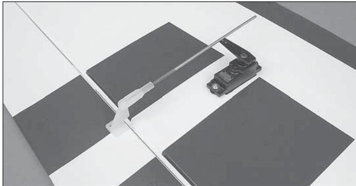
❑❑ 6. Cut the control horn and mounting plate apart. Attach the clevis in the outer hole of a nylon control horn. Place the control horn in line with the hole  $3/4$ " [19mm] from the center of the servo arm. When positioned properly the control horn will rest on a hardwood plate in the aileron. Mark the location of the mounting holes onto the aileron. Drill a  $3/32$ " [2.4mm] hole on the marks, drilling through the plywood plate and the top of the aileron.
