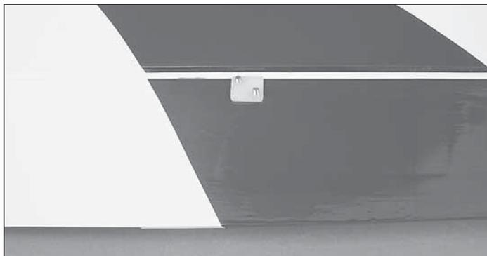
❑❑ 7. Insert two 2-56 x  $5/8$ " [16mm] machine screws through the control horn and aileron. Secure the control horn to the aileron with the nylon control horn backplate.
