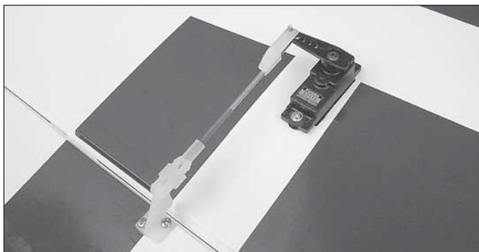
❑❑ 8. Slide a silicone clevis retainer over the clevis. With the aileron servo and the aileron centered, mark the aileron
