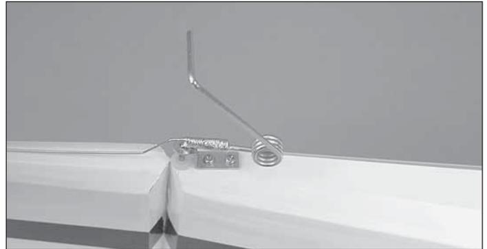
❑ 2. Insert the tail gear wire through the aluminum tail gear bracket. Insert the tail gear wire and bracket in the tail gear bushing. With the tail gear bracket aligned with the bottom of the fuselage, mark and drill a 1/16" [1.6mm] pilot hole at both tail gear bracket mounting hole locations. Secure the tail gear bracket to the fuselage with two 2 x 12mm sheet metal screws.
