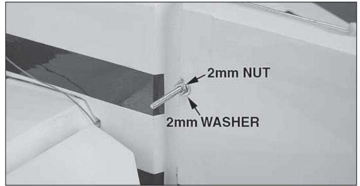
❑ 5. Insert the 2mm threaded rudder control horn rod. Center the rod in the rudder with two 2mm flat washers and 2mm nuts on each side. A drop of threadlocker on the threads will help prevent the nuts from coming loose.
