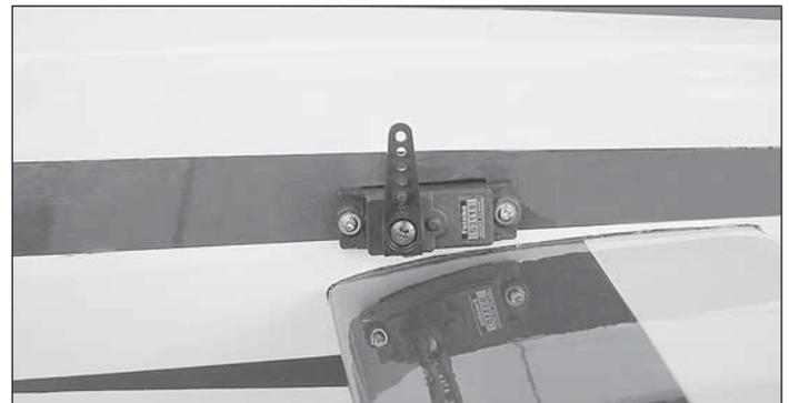
❑ 3. Install the rudder servo into the servo opening. Drill through the servo mounting holes with a 1/16" [1.6mm] drill bit. Remove the servo from the servo opening. Install and then remove a servo mounting screw into each of the holes you have drilled. Apply a drop of thin CA into the holes to harden the threads. Once the glue has hardened install the servo into the servo opening using the 2 x 7 x 9mm servo retaining plates. Center the servo, and then install a servo arm as shown.
