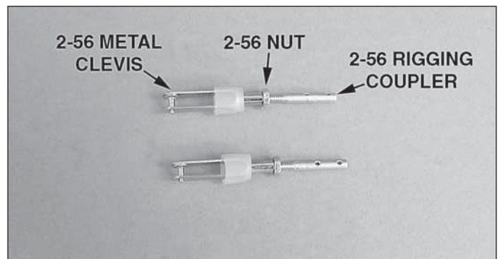
❑ 7. Thread 2-56 nuts onto four 2-56 rigging couplers. Slide a silicone clevis retainer over four threaded 2-56 metal clevises. Then, thread the clevises 10 turns onto the rigging couplers. Tighten the 2-56 nuts against the metal clevises.
