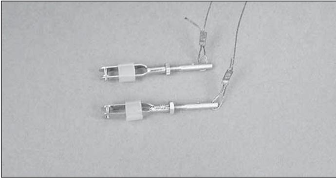
❑ 8. Working from the end of the string inside the fuselage, pass the string through a crimp, through the rigging coupler and back through the crimp. Squeeze the crimp with a pliers to secure the string in the crimp. Apply a drop of thin CA to the crimp.
