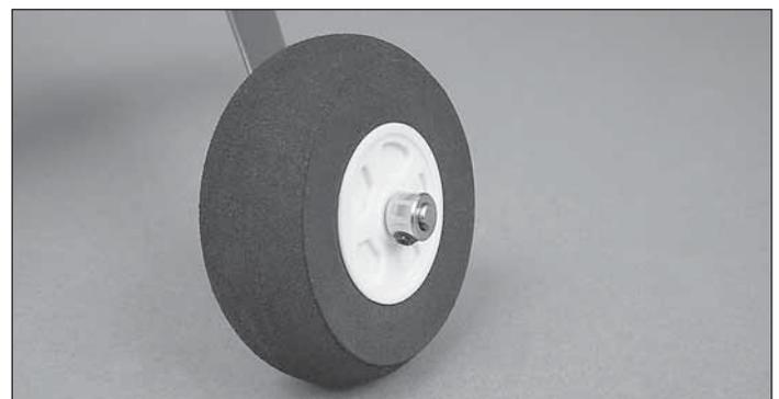
❑❑ 2. Install two 5mm flat washers on the axle, then the foam main wheel, followed by a 4.2mm wheel collar. Secure the wheel collar on the axle with 6-32 set screw. Mark the
