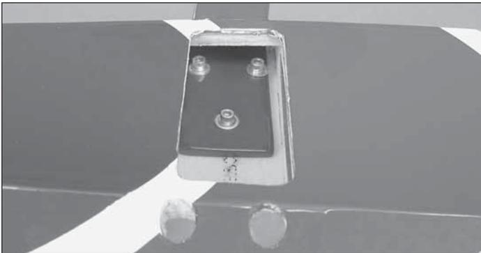
❑ 4. Attach the main landing gear to the fuselage with three 4-40 x 1/2" [12.7mm] SHCS, 3mm lock washers and 3mm flat washers.
