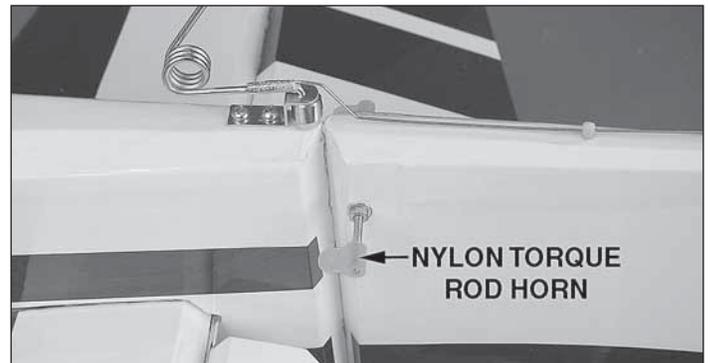
❑ 6. Thread a nylon torque rod horn onto each end of the control horn rod. Adjust the torque rod horn so that they are both equal distance from the rudder.
