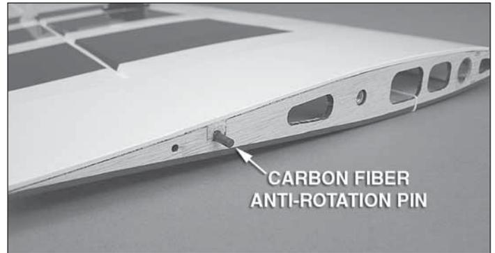
❑❑ 9. Glue the carbon fiber anti rotation pin in the hole as shown. The pin should protrude approximately  $1/4$ " [6.4mm].
