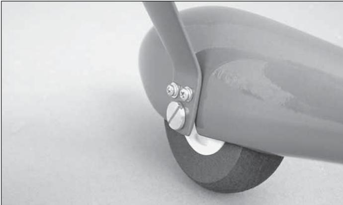
❑ 3. Position the right wheel pant over the wheel and secure it to the main landing gear with two 2-56 x 3/8" [9.5mm] machine screws, 2mm flat washers and 2mm lock washers.
