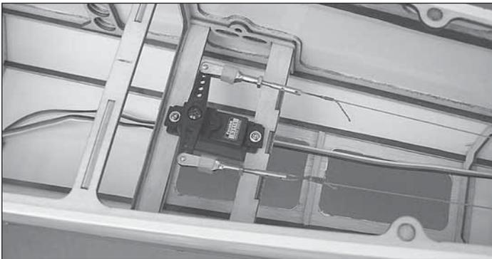
❑ 9. Attach the clevises to the rudder servo horn in the holes 3/4" [19mm] from the center.
