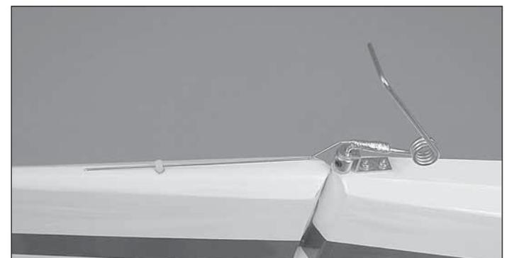
❑ 3. Thread a 4-40 set screw into the 2.5mm wheel collar. Remove the tail gear wire from the tail gear bracket and position the 2.5mm wheel collar under the bracket. Slide the
