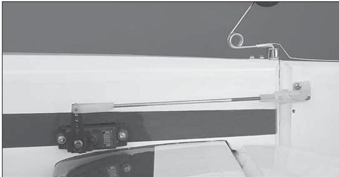
❑ 5. Slide a silicone clevis retainer over the clevis. With the rudder servo and the rudder centered, mark the rudder pushrod where it crosses the rudder servo arm. Make a 90° bend at the mark. Cut the pushrod 3/8" [9.5mm] past the bend. Attach the pushrod to the rudder servo arm with a nylon FasLink.
