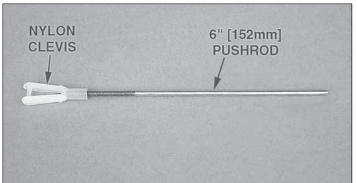
❑ 5. Thread a nylon clevis, 20 turns, onto a 6" [152mm] wire pushrod.
