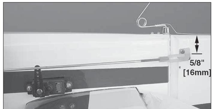
❑ 4. Thread a nylon clevis 16 turns onto a 2-56 x 6" [150mm] wire pushrod. Connect the clevis to the second hole from the base of a nylon control horn. Using the rudder pushrod, position the control horn in line with the servo arm.
