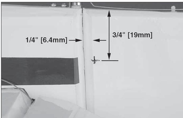
❑ 4. Measure up 3/4" [19mm] from the bottom of the rudder and make a mark. Measure in from the leading edge 1/4" [6.4mm] and make a mark. Drill a 3/32" [2.4mm] hole through the rudder, perpendicular to the centerline of the rudder.
