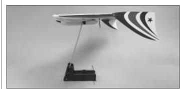
□ 2. Lift the model, upside down, at the balance point you marked on the top of the wing. In the photo, we are using a Great Planes CG Machine<sup>TM</sup>. If the nose drops the model is nose-heavy and you must add weight to the tail. If the tail drops, the model is tail-heavy and you must add weight to the nose. In most cases you can relocate the receiver to achieve the correct balance without adding more weight.
