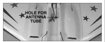
□ 1. Remove the pushrods from the control horns. Insert the pushrods through the holes in the center section. Route the servo wires through their respective holes. Position the center section onto the wing and check that the hole for the receiver antenna is aligned with the antenna tube in the left wing panel. Adjust the hole in the center section as needed.
