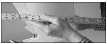
$\Box$  2. Check the ailevators to see if they are centered. Use a straightedge to align the bottom of the ailevators with the bottom of the wing as shown above. If necessary, adjust the clevises on the pushrods to center the ailevators.
