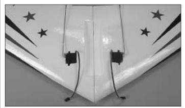
$\Box$  2. Join the right wing panel onto the joiner tubes in the left panel. Use the white tape on the bottom of the wing to hold the wing panels together.
