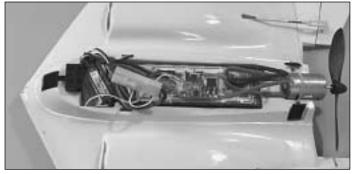
□ 2. Fit the canopy (battery cover) to the center section. The ESC can be held to the top of the battery with some Velcro tape.
