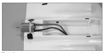
□ 3. Secure the motor to the center section with the included nylon tie strap. Notice that the wires have already been soldered to the motor.
