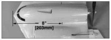
□ 1. Use a felt-tip pen or narrow strips of tape to mark the balance point on the **top** of the wing 8" [203mm] from the forward most part of the model.
