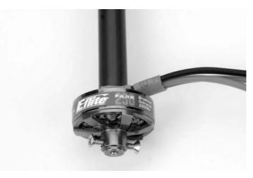
**NOTE:** Photo shows installation using a carbon fiber tube, with 8mm OD, 6mm ID (EFLM1960 available separately). This is an option for mounting the motor. You can cut down the carbon fiber tube to meet your specific needs and attach to your foam or wood airplane with glue.
