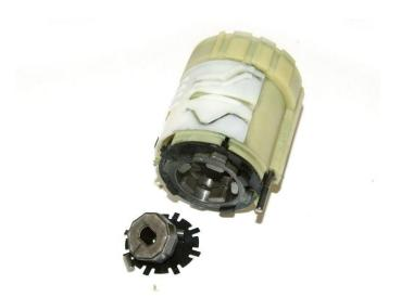
Remove and discard the roller pins, the 5-sided output coupler, and the black steel shim. Reinstall the black plastic cover in the same orientation it was removed from. After this step, the output of the transmission will be a 5-sided socket.
