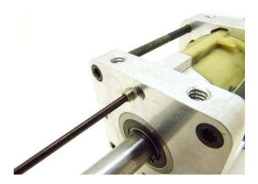
Using a 3/32" hex wrench, screw in the #10-32 x ¼" set screw into the off-center hole found on the front of the output assembly. As you tighten the screw, the torque clutch plunger will begin moving.
