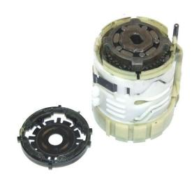
Remove the black plastic front cover from the 397892 transmission by gently bending the two clips molded into the casing. The five anti-backdrive roller pins and 5-sided output coupler will be visible.
