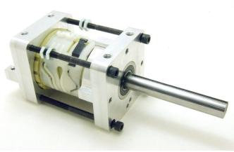
Insert the 4 #10-32 x 3" screws into the output assembly holes, but do not tighten yet. Thread on two #10-32 machine hex nuts onto the top **two** screws nearest to the gear selector, spaced ½" from the end of the screw.
