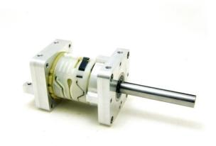
Using gentle pressure, push the rear of the transmission into the mount. Approximately 1/8" of the rear portion of the transmission will be visible.
