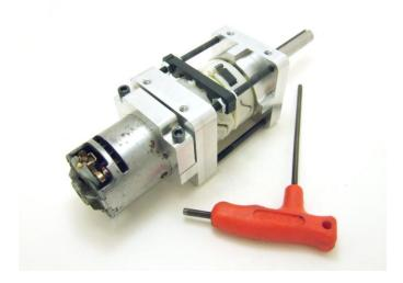
Finally, install the motor clamp ring and the two #10-24 x 1.5" screws using a 5/32" hex wrench. Take care to tighten the screws evenly, and do not exceed more than ¼ turn per screw from a hand-tight position. When fully tightened, the gap between the motor clamp ring and the transmission mount is approximately 0.025".
