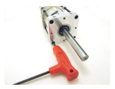
Use a 5/32" hex wrench to tighten the face mounting screws. To maintain squareness, do not tighten one screw "all the way" first.
