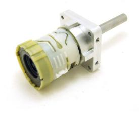
Gently push the transmission into the output assembly while rotating the output shaft with your hand to line up the output spline with the 5-sided output socket.
