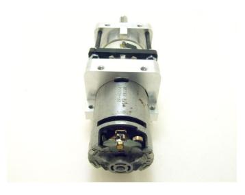
With the crimps adjusted, slide the motor into the rear transmission mount. Rotate the motor slightly to engage the planetary gears. Push in the motor until the forward case vents are barely flush with the face of the rear transmission mount, as shown. The motor can be installed in any orientation.
