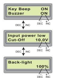
The beep sounds at every time pressing the buttons to confirm your action. The beep or melody sounded at various times during operation to alert different mode changes. These audible sounds can be on or off.
