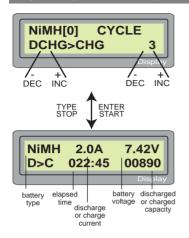
Set the sequence on the left and the number of cycle on the right. You can use this function for balancing, refreshing and break-in the battery. To avoid rising temperature of the battery, there will a brief cool-off period that already fixed at 'User program setup' after each charge and discharge process.
