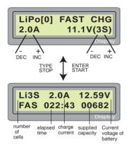
You can set up the charging current and the voltage of the battery pack being charged. As you press 'ENTER/START' button the voltage confirmation will be displayed. And then, if you confirm the voltage and current, press 'ENTER/START' button again to start charging.
