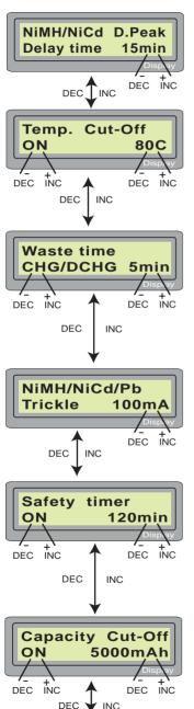
This restrains the delta-peak voltage detection until the time has reached. This prevents a premature cut-off from the battery of high internal resistance. The default value is one minute. (1  $\sim$  15 minutes)
