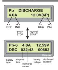
Set discharge current on the left and final voltage on the right. The discharge current ranges from 0.1 to 7.0A.
