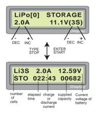
You can set up the current and the voltage of the battery pack to be charged. The current will be used for charge or discharge the battery to reach the 'storage' level of voltage.
