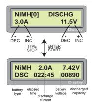
Set discharge current on the left and final voltage on the right. The discharge current ranges from 0.1 to 7.0A and the final voltage ranges from 0.1 to 30.0V).
