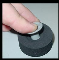
Next, simply push the wide-hub half of the wheel back into the tire. Either side, it doesn't matter.
