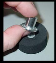
Now flip over the wheel and align the new aluminum hub on the other side of the wheel so that the threaded hole in the center lines up with the center of the wheel.
