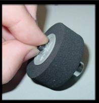
Insert the screw through the plastic side of the wheel and thread it into the aluminum hub on the other side.
