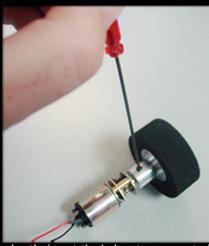
Lastly, insert the hub onto your motor's output shaft and tighten down the set screw (preferably onto the shaft's flat, if there is one).
