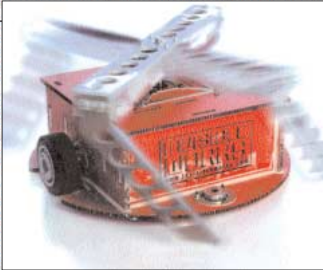
Snipe is a lightweight robot made out of mostly composite material. Creator Charles Habermann cut many of Snipe's parts on a 5-axis, 55,000-psi waterjet cutting system.
